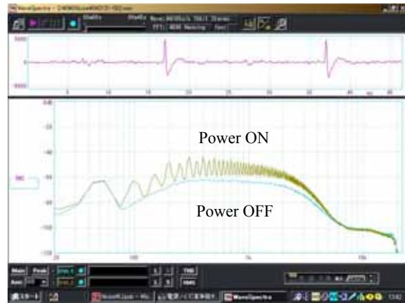
Radiated noise from power cable of a massage chair (power ON and power OFF)
