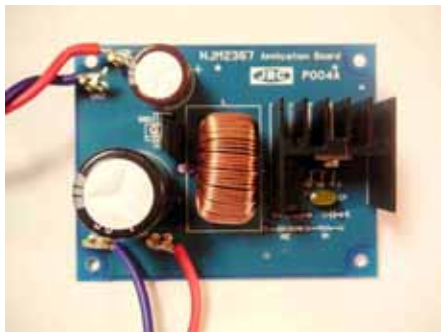
NJM2367 Step Down DC-DC Converter Evaluation Board
